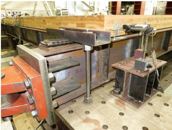
(c) 振れ止めの状況 [加力側]
