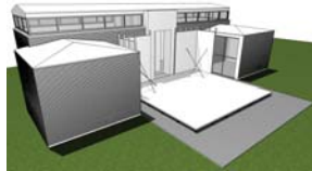
step 3: ribbed wall elements and temporary securing
