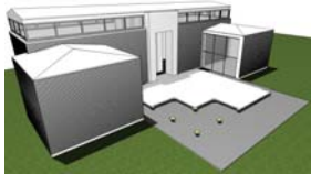
step 2: CLT floor elements
