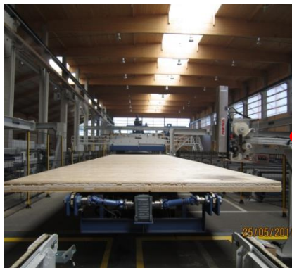
CLT element ready for cutting and joining
