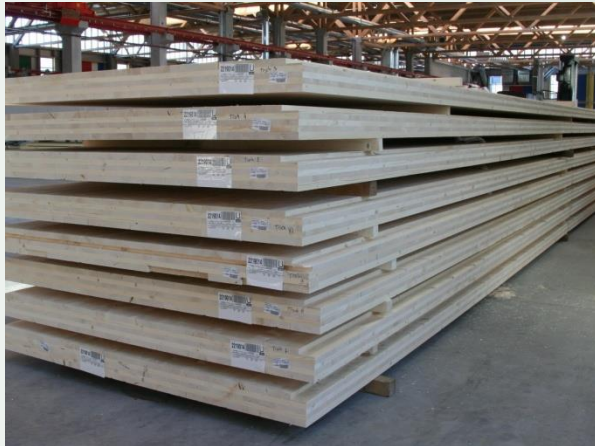
storage of CLT elements (production site)
