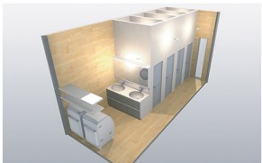
CLT SANITARY UNIT
